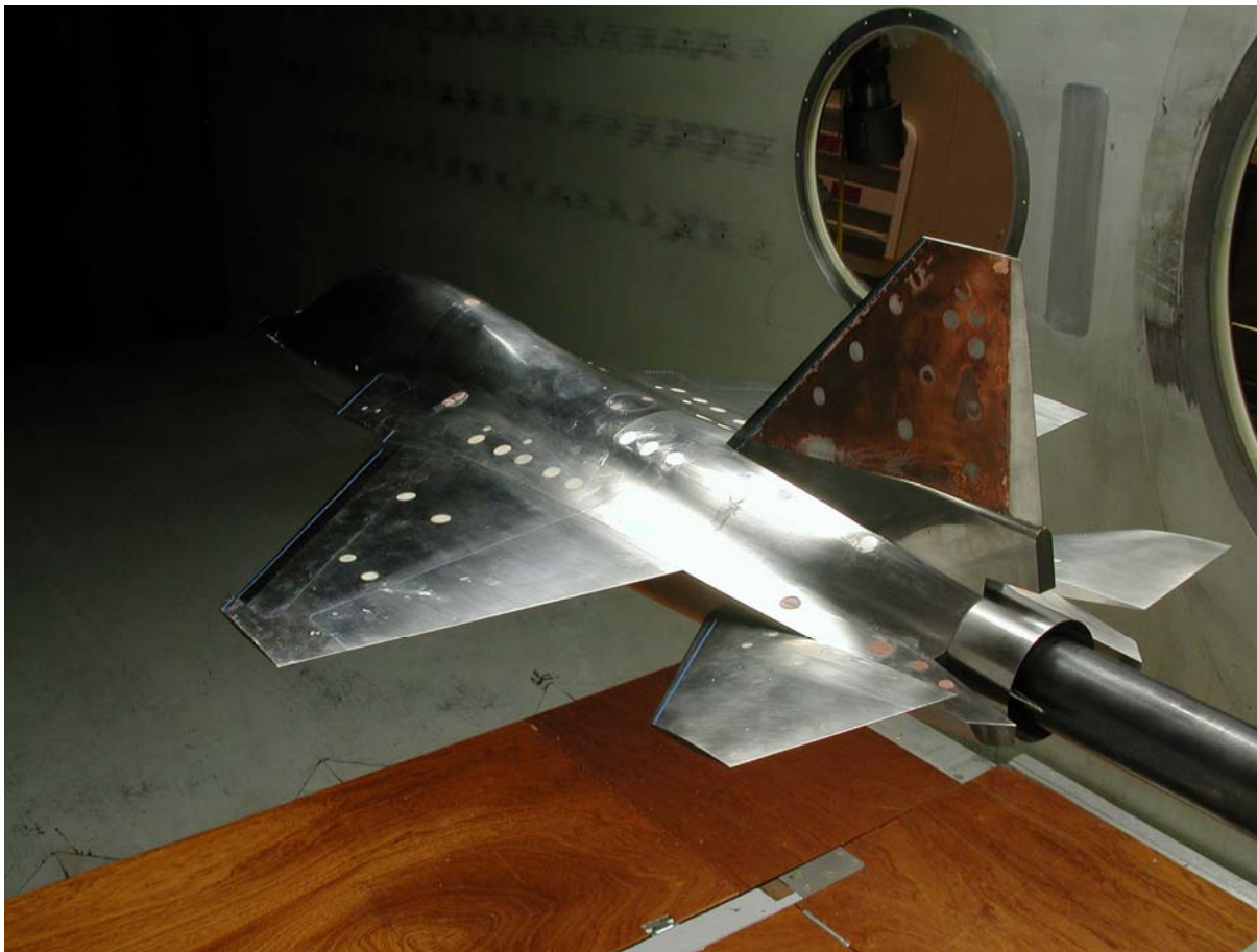
Figure 3: Model in NLR HST wind tunnel – Fin instrumented with PVDF foil
